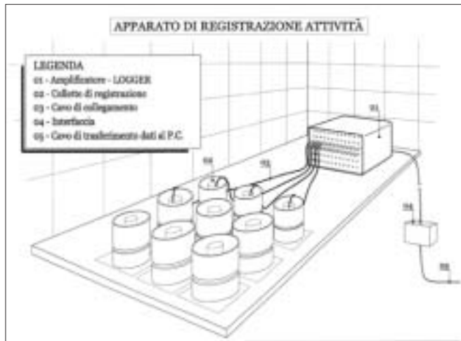
FIG. 3.4.4 Recording chambers used for the analysis of activity rhythm of Talitrus saltator . A single animal was added to each chamber, which was then covered with a sheet of polythene, secured by a rubber band. 01. Amplifier – logger; 02. Recording chambers; 03. Connection to the interface; 04. Interface; 05. Connection to the PC outside the controlled environment cabinet
